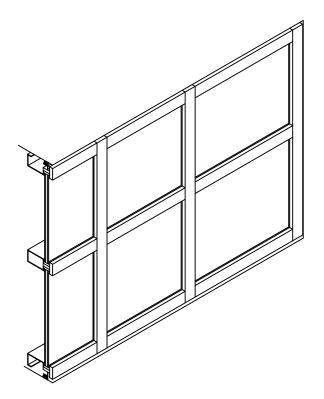
Graham 2505C series curtainwall is an outside glazed captured system designed for low to medium rise structures. It has a face width of 2 1/2" and a depth of 5 1/4". It incorporates a split male-female vertical mullion which allows factory assembly and sealing of the frame.
