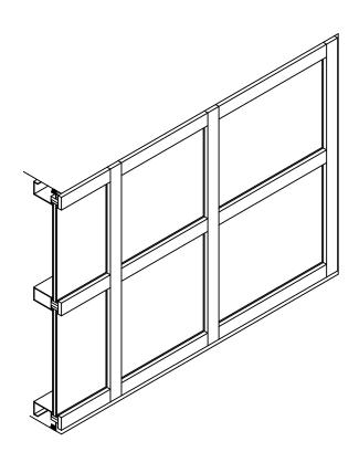
Graham 2506C series curtainwall is an outside glazed captured system designed for low to medium rise structures. It has a face width of 2 1/2" and a depth of 6 1/4". It incorporates a split male-female vertical mullion which allows factory assembly and sealing of the frame.
