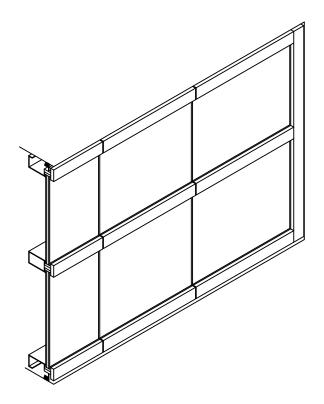
Graham 2506S series curtainwall is an outside vertically butt glazed system designed for low to medium rise structures. It has a face width of 2 1/2" and a depth of 6 1/4". It incorporates a split male-female vertical mullion which allows factory assembly and sealing of the frame.
