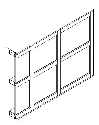
Graham 2507C series curtainwall is an outside glazed captured system designed for low to medium rise structures. It has a face width of 2 1/2" and a depth of 7 1/4". It incorporates a split male-female vertical mullion which allows factory assembly and sealing of the frame.
