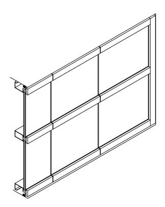
Graham 2507S series curtainwall is an outside vertically butt glazed system designed for low to medium rise structures. It has a face width of 2 1/2" and a depth of 7 1/4". It incorporates a split ale-female vertical mullion which allows factory assembly and ealing of the frame.
