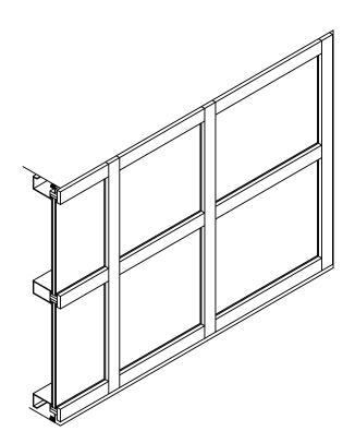
Graham 2508C series curtainwall is an outside glazed captured system designed for low to medium rise structures. It has a face width of 2 1/2" and a depth of 8 1/4". It incorporates a split male-female vertical mullion which allows factory assembly and sealing of the frame.
