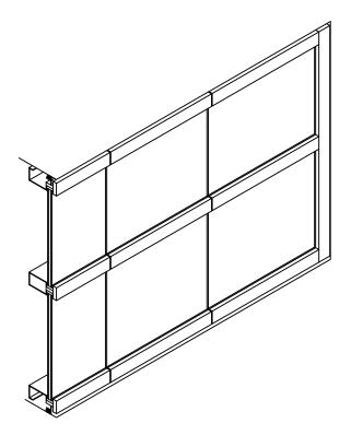
Graham 2508S series curtainwall is an outside vertically butt glazed system designed for low to medium rise structures. It has a face width of 2 1/2" and a depth of 8 1/4". It incorporates a split male-female vertical mullion which allows factory assembly and sealing of the frame.
