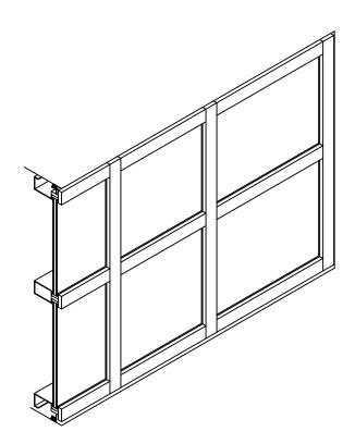
Grraham 2510C series curtainwall is an outside glazed captured system designed for low to medium rise structures. It has a face width of 2 1/2" and a depth of 10 1/4". It incorporates a split male-female vertical mullion which allows factory assembly and sealing of the frame.
