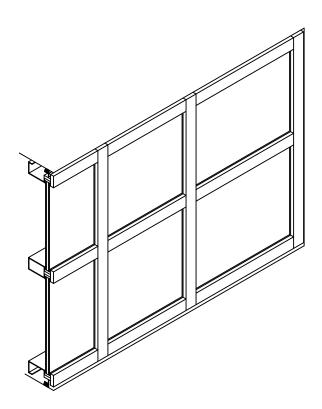
Graham 3010C series curtainwall is an outside glazed captured system designed for low to medium rise structures. It has a face width of 3" and a depth of 10 1/4". It incorporates a split male-female vertical mullion which allows factory assembly and sealing of the frame.
