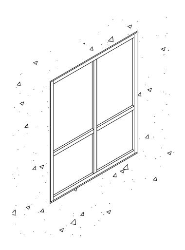
Graham 450T series window is an inside glazed system designed for punched and strip window applications. The overall frame size is 2" wide and 4 1/2" deep. This series incorporates an interior removable glazing bead at the top of each lite that allows for interior glazing.
