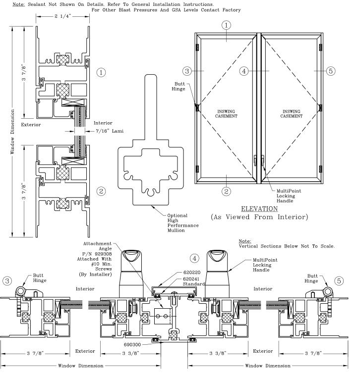
Note: Dashed Lines Represent Inswing Vented Units Solid Lines Represent Outswing Vented Units; Lines Converge At Hinge Side Of Vent
