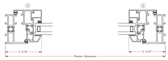
Note: Dashed Lines Represent Inswing Vented Units Solid Lines Represent Outswing Vented Units; Lines Converge At Hinge Side Of Vent
