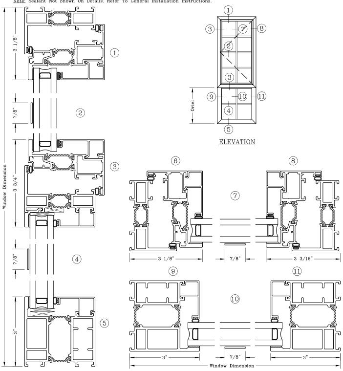
Note: Dashed Lines Represent Inswing Vented Units Solid Lines Represent Outswing Vented Units; Lines Converge At Hinge Side Of Vent Graham Architectural Products reserves the right to change, add, cancel, remove or otherwise modify the details illustrated without prior notice.
