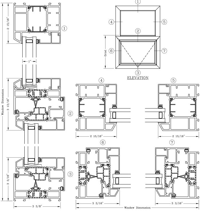
Note: Dashed Lines Represent Inswing Vented Units Solid Lines Represent Outswing Vented Units; Lines Converge At Hinge Side Of Vent Graham Architectural Products reserves the right to change, add, cancel, remove or otherwise modify the details illustrated without prior notice.
