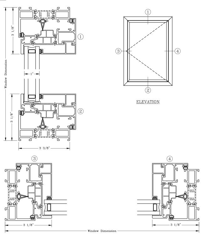
Note: Dashed Lines Represent Inswing Vented Units Solid Lines Represent Outswing Vented Units; Lines Converge At Hinge Side Of Vent
