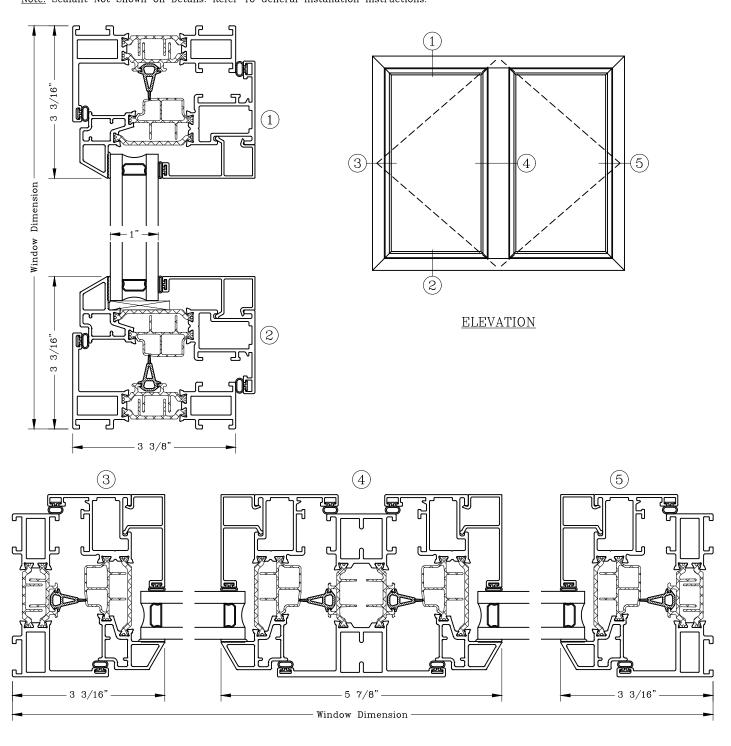
Note: Dashed Lines Represent Inswing Vented Units Solid Lines Represent Outswing Vented Units; Lines Converge At Hinge Side Of Vent
