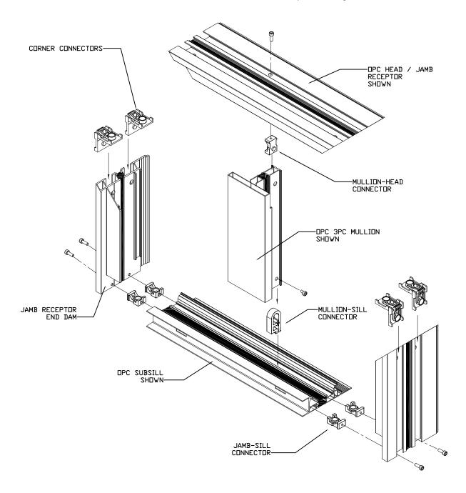
NOTE: THIS RECEPTOR SYSTEM IS FACTORY FABRICATED.
