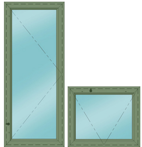
Note: Phantom line represents inswing impact panel operation for cleaning and blind access. Lines converge at hinge side of panel.
