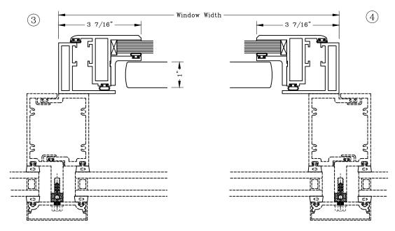
Note: Dashed Lines Represent Inswing Vented Units Lines Converge At Hinge Side Of Vent
