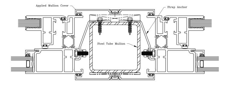
Details Shown Are For Concept Proposal Only Contact Graham Architectural Products For Job Specific Installation Anchoring Proposal Details Based On Building Conditions
