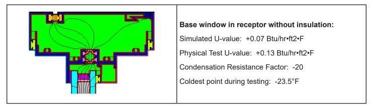
Adding insulation to the perimeter of the receptor system improves this scenario significantly. The U-value reduced by 0.06 BTU/ft<sup>2</sup>/hr, the CRF improved by 11 points and the lowest interior frame temperature was 14 degrees warmer when compared to the non-insulated window in receptor. This is an improvement in thermal performance when compared to the window in receptor without insulation. The thermal performance is similar to the window by itself.
