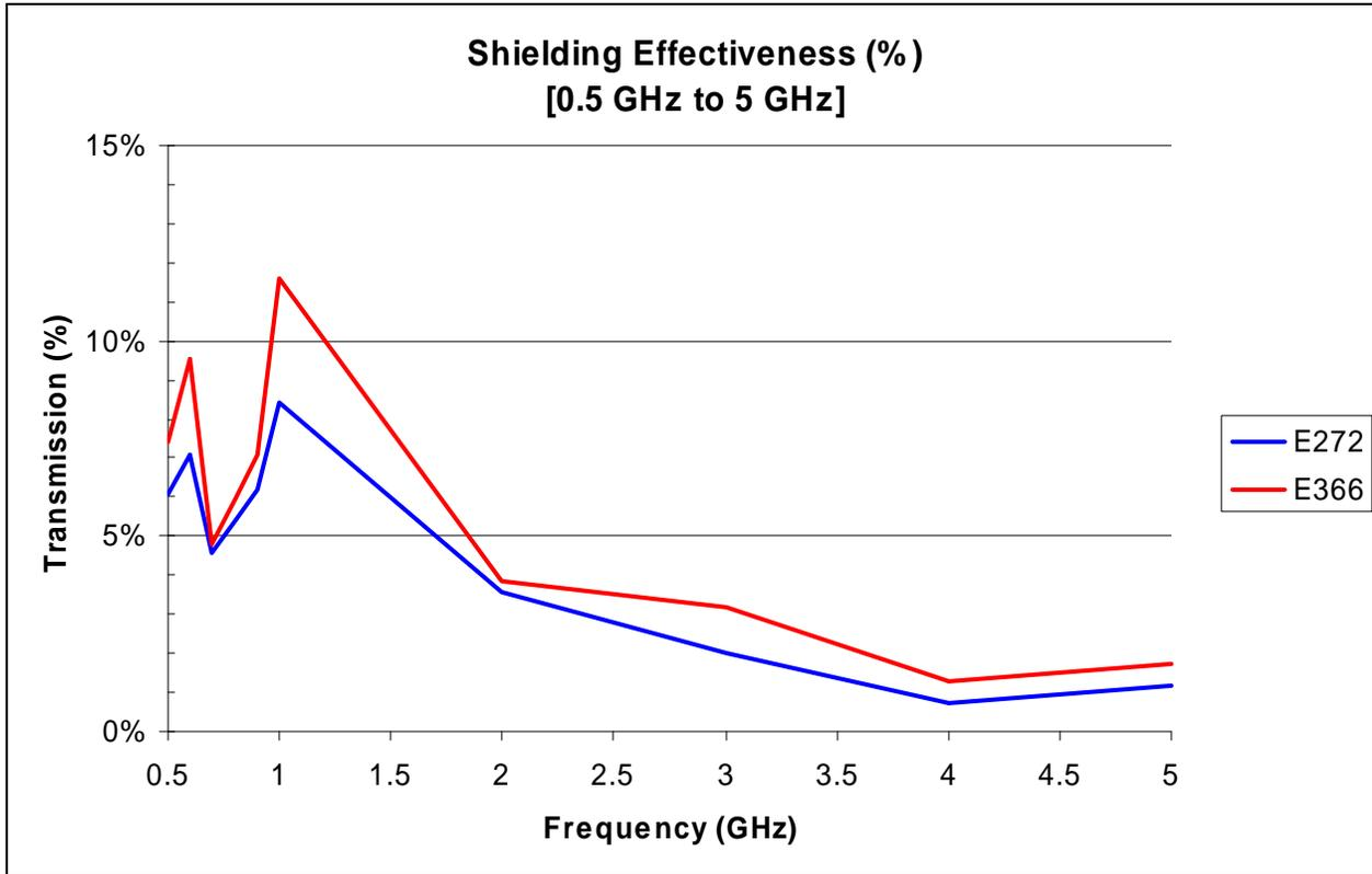
The measurements on Cardinal CG samples agree with the literature numbers quite well, although the numbers are not directly comparable because the measurements cover different portions of the spectrum. The fact that the E272 sample shields slightly more effectively than the E366 sample is a little surprising and no reason can be offered at this time.
